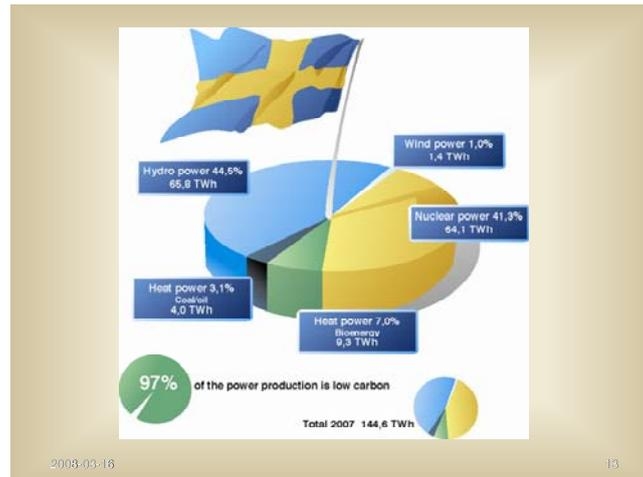
As you can see on the picture almost 90 % of Sweden's electricity is produced from hydro power and nuclear power, with both producing about equal amounts. The remainder is produced by fossil power, biofuels and wind power. Thus, power production is almost carbon dioxide-free in Sweden.
